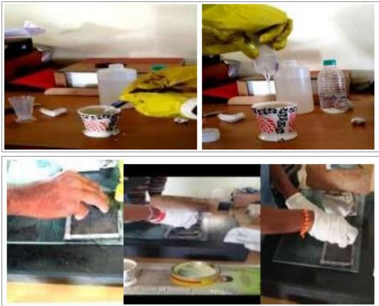
Figure 2: Preparation of Samples for CFRP
