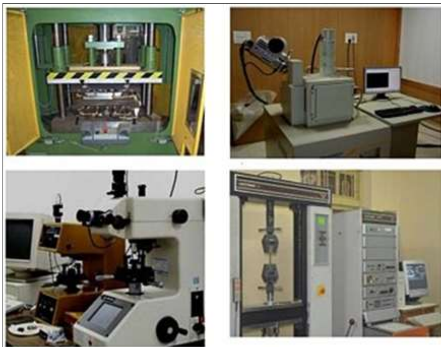
Figure 5: Testing Equipment Includes a Compression Molding Machine, Scanning Electron Microscope, Leitz Micro Hardness Tester, and Instron 1195 Universal Testing Machine
