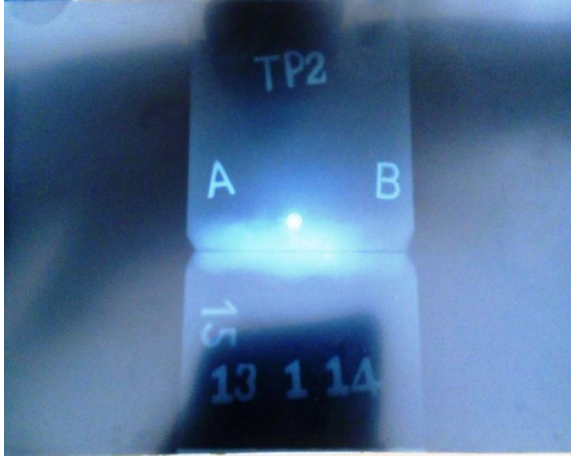
Fig 9: Radiography Test Result on Cold Crack Specimen
