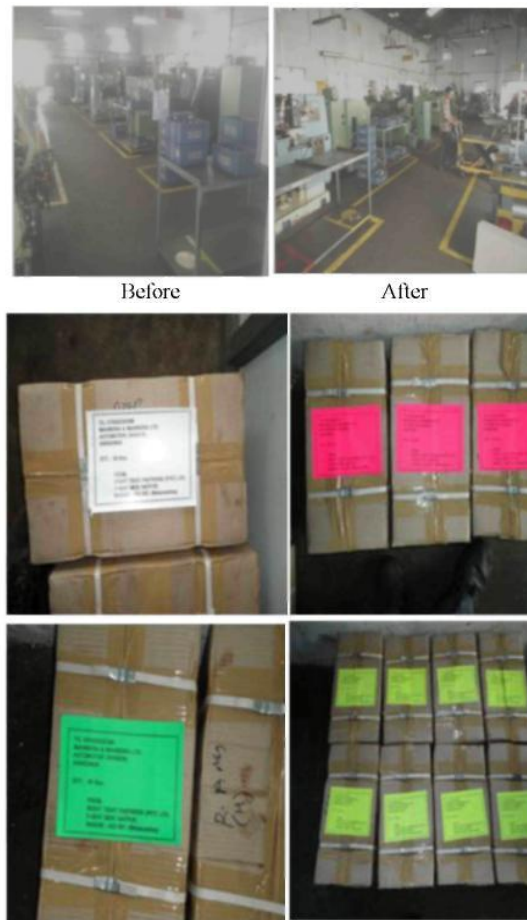
Fig 10: Marking and Standardization of the Templates with different color codes, (each color code specifies a particular company/product which helps in minimizing the problem of dispatching the different product to other company).
