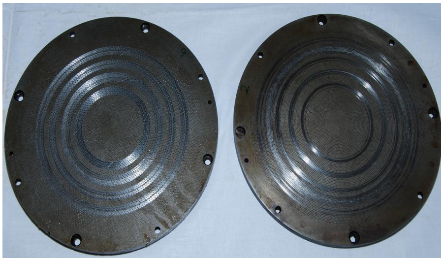
Fig 4b: Disc with Worn Track
