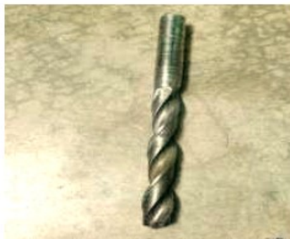
Figure 4: (a) (Single Coated) HSS Drill Bit with TiAlN, (b) Figure.4. (Double coated) HSS Drill Bit with TiAlN
