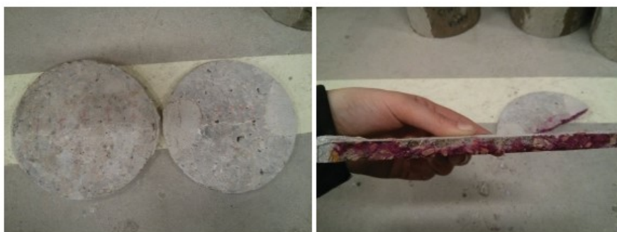
Figure 12: Sealed Disks (Left) and Broken Half of a Disk After the Phenolphthalein Test (Right)
