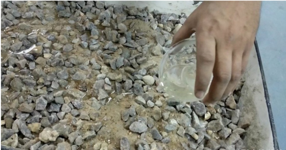
Figure 4: Mixing of PCM in Liquid State
