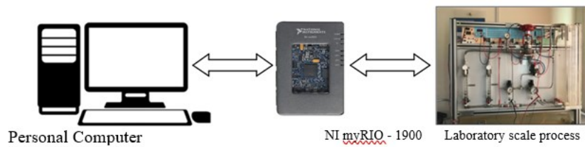
Figure 5: Block Diagram for Process Dynamics Estimation
