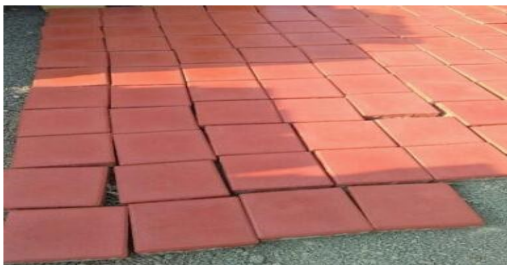
Figure 6: Cast Paver Block for Various Proportions of Waste Bakelite
