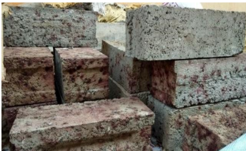
Fig 5: Cast Solid Block for Various Proportions of Waste Bakelite
