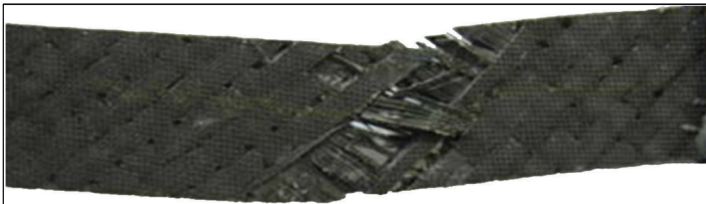
Figure 10: Shear Tested Specimen of Multiscale composite.
